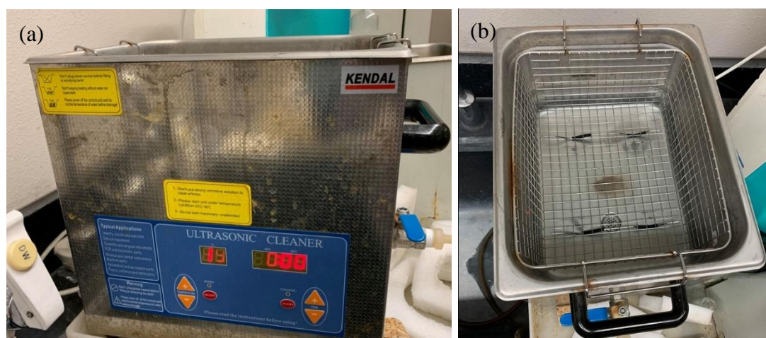
Figure 3.5 (a-b) An ultrasonic cleaner from Kendal corporation.
